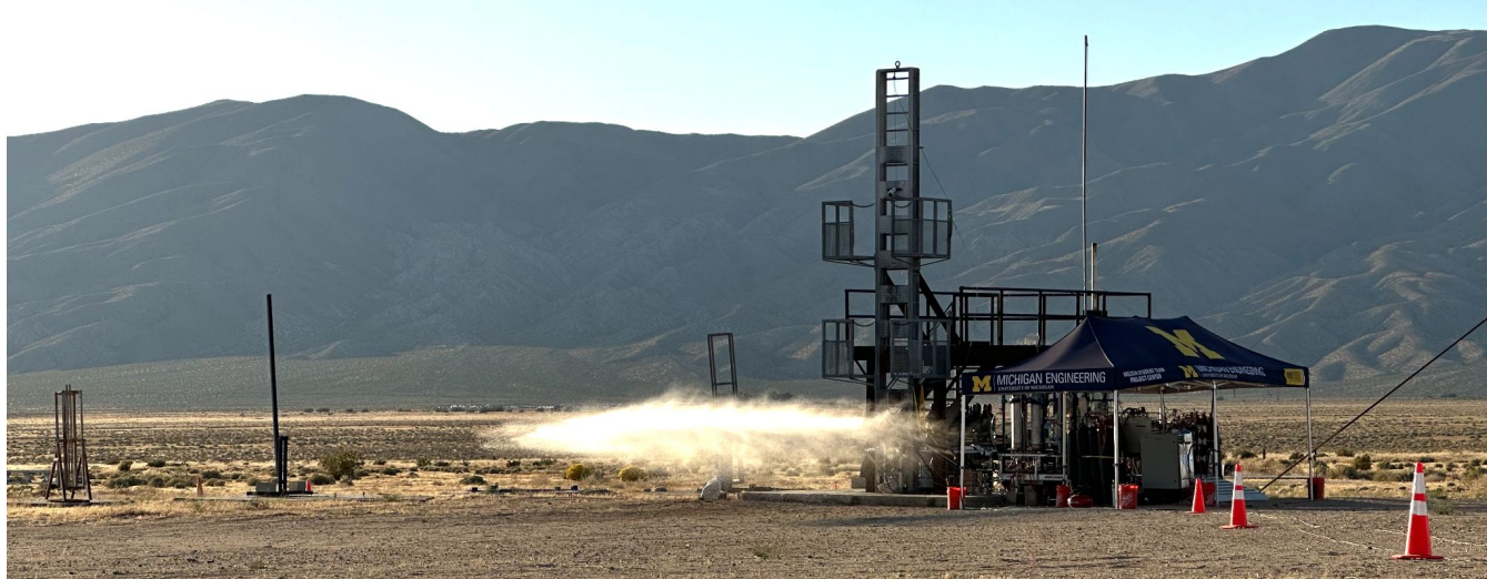
Inert propellant flow test of MASA's ME-5 Engine – May 2024
